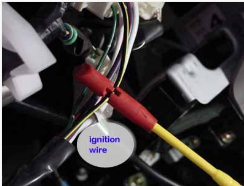
Wiring Photo and Notes: Second Ignition
