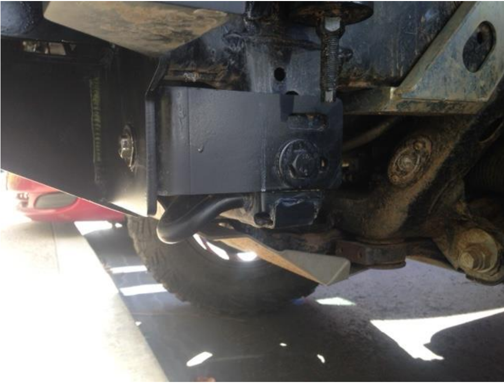
Reinforcement Bracket Installed
