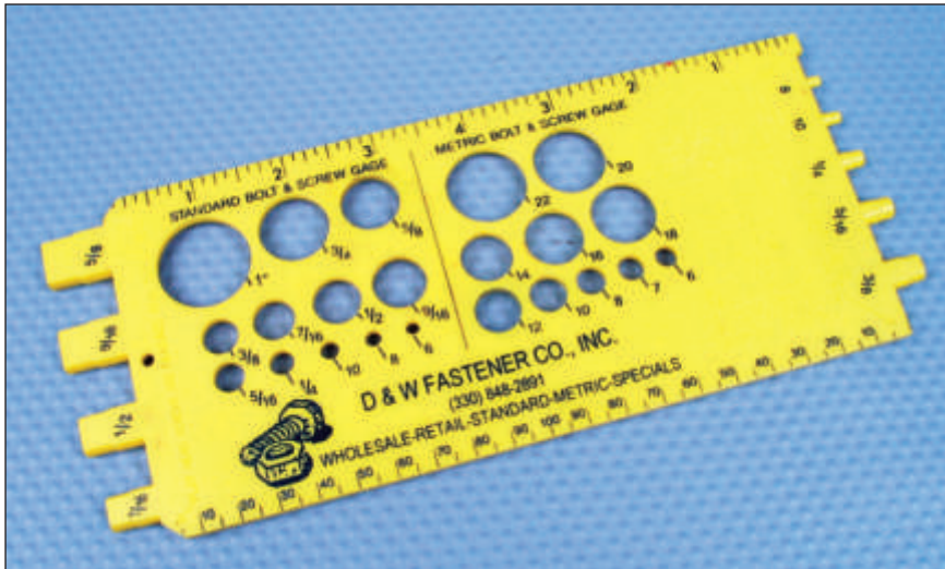
Fastener sizing cards are handy to determine bolt or stud diameter (both inch and metric), as well as bolt or stud shank lengths and nut diameters.
