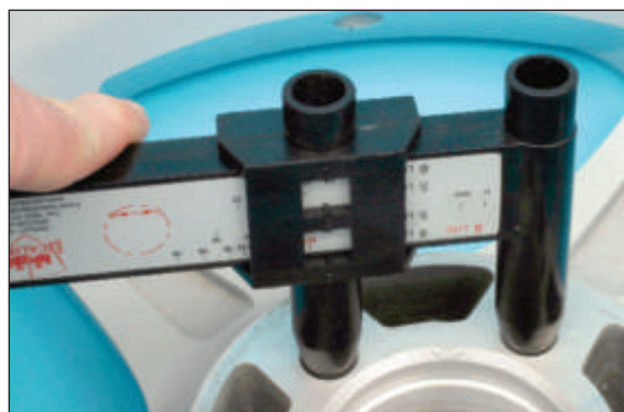
This handy caliper-style tool can be used to quickly determine bolt circle. Insert both pins into adjacent holes and read the gauge.
