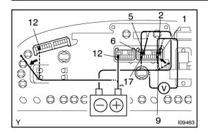
(d) Check that the voltage of the terminals 5 and 6 of the connector "D" is 0 V after terminal 12 of the connector "C" has been disconnected and terminal 9 of the connector "D" has been connected to the negative (–) lead from the battery.
