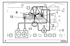
(e) Check that the voltage of the terminals 5 and 6 of the connector "D" is battery positive voltage after terminals 1 and 2 of the connector "D" has been disconnected and reconnected.
