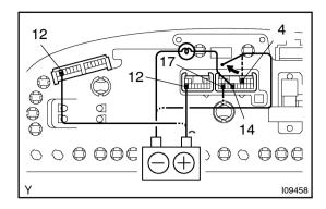
(g) Check that the buzzer stops sounding when disconnecting terminal 4 from the negative (–) lead.
