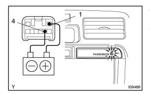
**30. INSPECT PASSENGER SEAT BELT WARNING LIGHT** Connect the positive (+) lead from the battery to the terminal 1 and negative (-) lead to terminal 4, and check that the warning light lights up.
