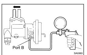
(b) Check that the sleeve fork moves away from the actuator when a vacuum of 66.7 kPa (500 mmHg, 19.69 in.Hg) is applied to port B. Also check that the vacuum remains constant.
