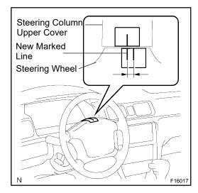
(d) Turn the steering wheel to its straight position. HINT:
