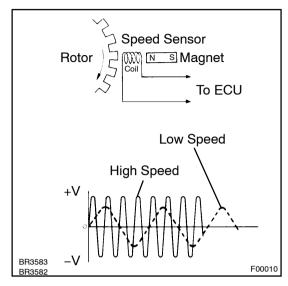
The speed sensor detects wheel speed and sends the appropriate signals to the ECU. These signals are used to control the ABS system. The front and rear rotors each have 48 serrations.
