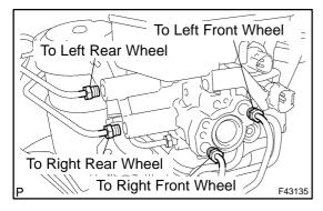
(b) Using SST, connect the 4 brake lines to the correct position of brake master cylinder as shown in the illustration. SST 09023-00100
