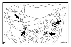
(b) Using SST, disconnect the 4 brake lines from brake master cylinder.
