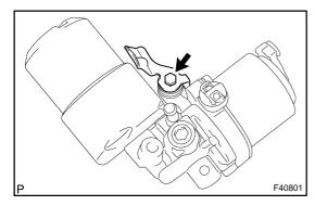
(b) Install the brake booster pump bracket with the bolt.
