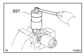
(b) Using SST, install the brake booster accumulator assy. SST 09318-12010
