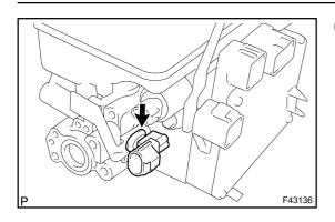
(b) Install the brake fluid level warning switch connector to the brake actuator bracket No.1.
