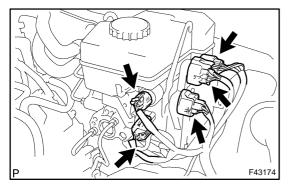
(c) Connect the 5 connectors to the brake master cylinder.
