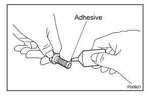
(b) Apply adhesive to 2 or 3 threads of the mounting bolt end. **Adhesive:**
