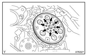
(b) Remove the 8 bolts, front spacer, drive plate and rear spacer.
