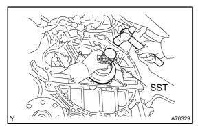
5. INSTALL ENGINE REAR OIL SEAL
