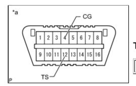
(4) Using SST, connect terminals 12 (TS) and 4 (CG) of the DLC3.
