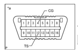
(2) Using SST, connect terminals 12 (TS) and 4 (CG) of the DLC3.
