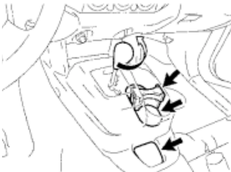
C. Automatic Transmission with bench seat. Remove shift knob by twisting counterclockwise.
