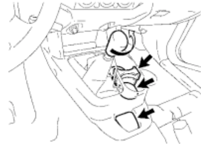
D. Manual transmission with bench seat. Remove shift knob by twisting counterclockwise.
