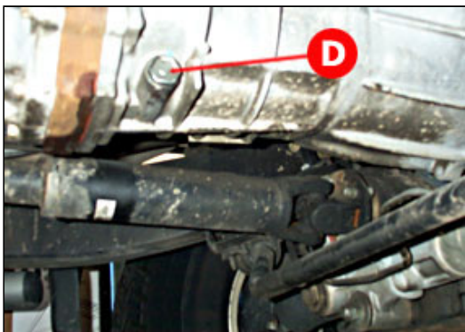
Remove the 24mm drain plug/washer. This one is very easy to remove.
