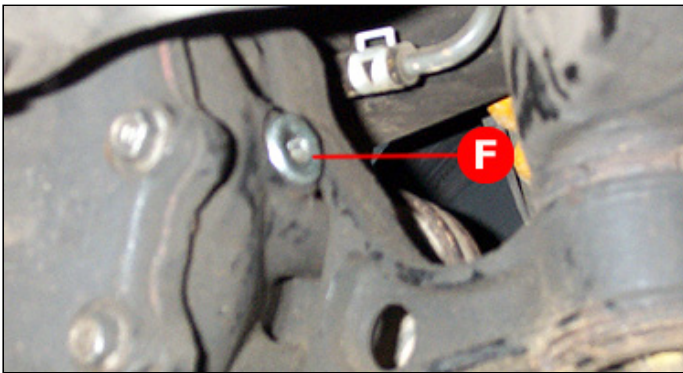
Remove the front differential drain plug w/ a 10mm hex. Excuse the blurry picture.
