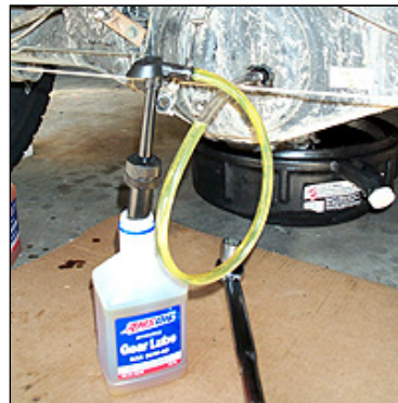
Pump 2.6 qts of gear lube in
