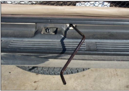
Lower the tire by cranking counter-clockwise
