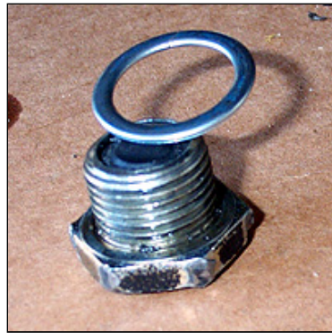
Clean off the magnetic drain plug
