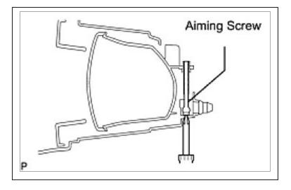
(a) Adjust the fog light aim into the specified range by turning the aiming screw with a screwdriver.
