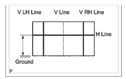
(e) Draw base lines (H line, V LH and V RH lines) on the screen as shown in the illustration.
