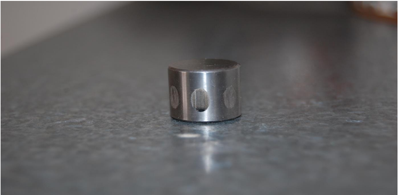
Picture 5: Reference Test Block with several scars from same oil
