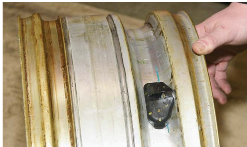
This photo shows a tire pressure monitor valve sub-assembly mounted to a wheel. Care must be taken during tire mounting/demounting to avoid sensor damage.
