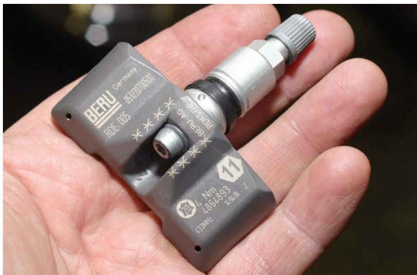
An example of a tire pressure monitor valve sub-assembly. This mounts to a drop area in the wheel.
